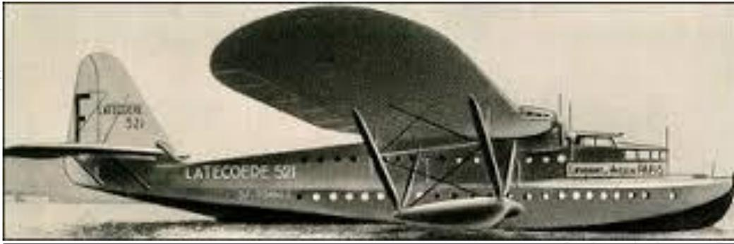
A single L.521 was built as a six-engine flying boat transport aircraft in 1935. The L.521 was designed for transatlantic flight and could fly non-stop from New York to Biscarrosse, on the French Atlantic Coast. This unit represents an expanded production and militarization of the L.521. Such an aircraft would have been fitted with depth charges and torpedoes for maritime duty.
