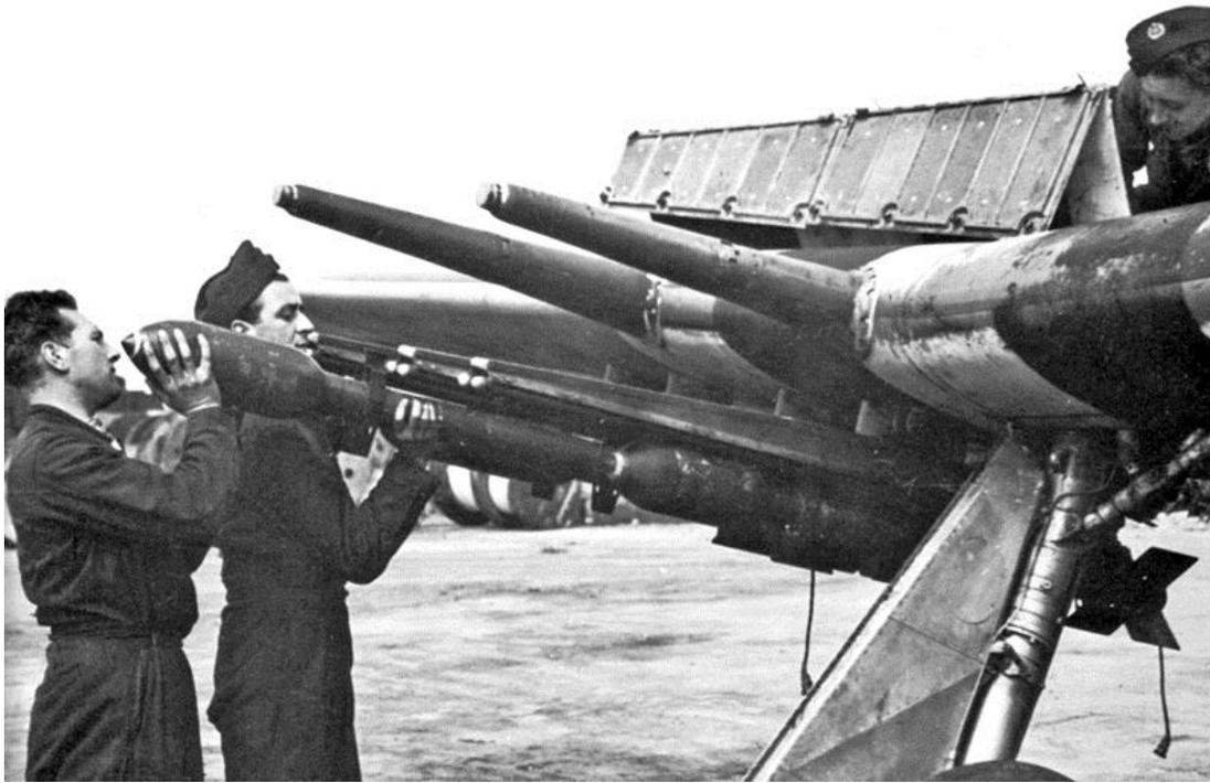
2.5 *RP-3 Rocket*: The RP-3 was an air-launched rocket. It was produced in 60lb high explosive and 25lb armor piercing variants. A 60lb SAP (semi-armor piercing) was introduced later in the war. RP-3 rockets were used effectively against submarines
